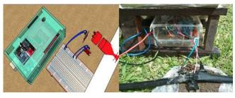
Figure 15 Xbee Transmitter
