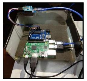
Figure 16 Xbee receiver
