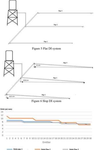
Figure 7 Flow rate (Debit) on flat DI system
