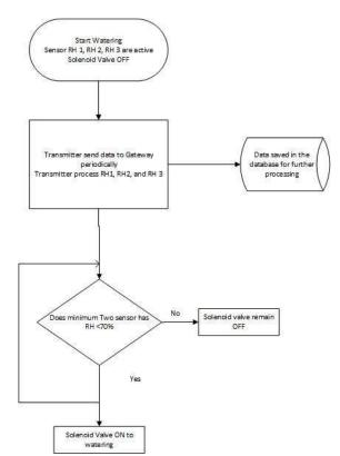
Figure 2 A flow chart of ON/OFF solenoid valve
