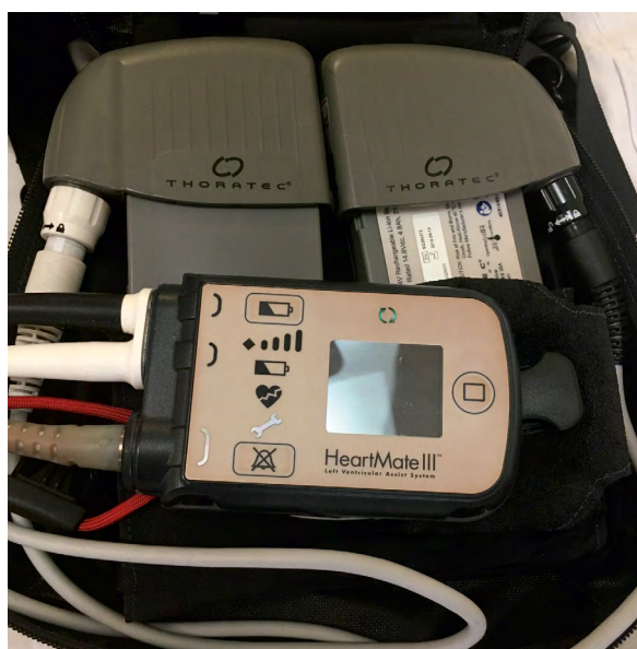
Figure 2. Left ventricular assist device (LVAD) controller and battery set
