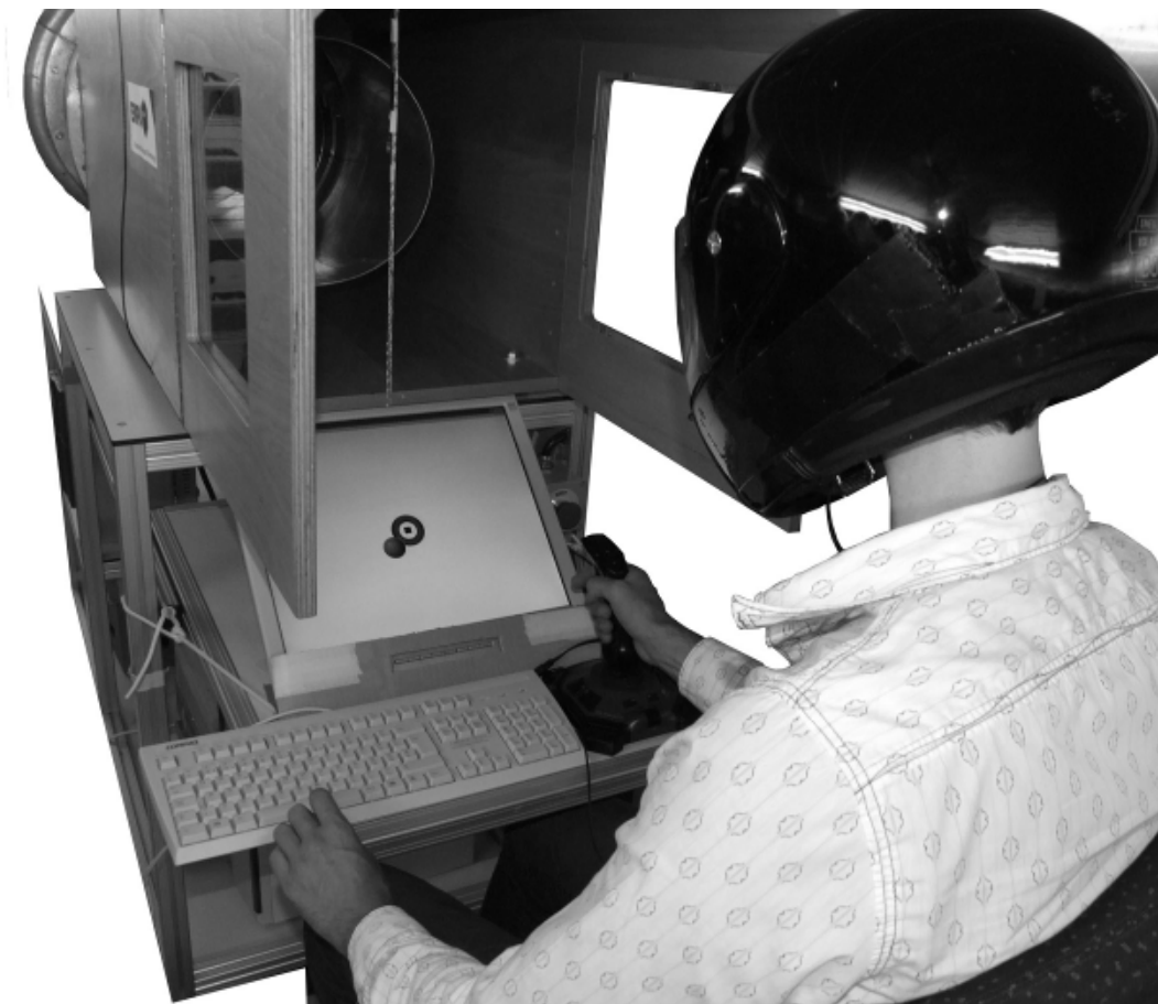
Figure 6.2: A subject during a pilot measurement, carrying out the simultaneous visual vigilance and tracking test (VTT) and auditory vigilance test (AVT); the screen shows the VTT. The AVT was experienced through the earphones.
