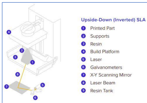
Figure 1: Diagram of Form2 SLA printer. Diagram is taken with permission from FormLab: Intro to Stereolithography 3D Printing.
