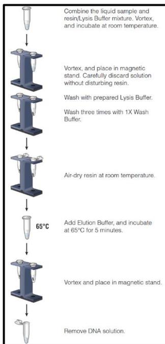
*Figure 1.3: DNA IQ™ System [55]. A schematic of the DNA IQ™ System with MagneSphere® Technology Magnetic Separation Stand. Silicon-coated paramagnetic resin is used to bind to DNA when in a high-salt solution. The MagneSphere® Technology Magnetic Separation Stand pulls the magnetic resin bound with DNA to the side of the tube while multiple washings take place to remove cellular components and purify the DNA.*
