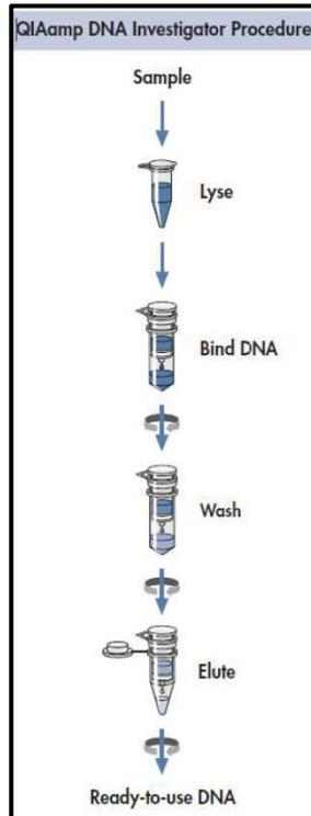
Figure 1.4: QIAamp<sup>®</sup> DNA Investigator Procedure [56]. A schematic of the Qiagen QIAamp<sup>®</sup> DNA Investigator Kit workflow. After lysing cells, the solution is added to a silica-based column that selectively binds DNA in a chaotropic salt solution. While bound, the DNA is washed using ethanol-based wash buffers before a low salt buffer is used to elute the DNA from the column.
