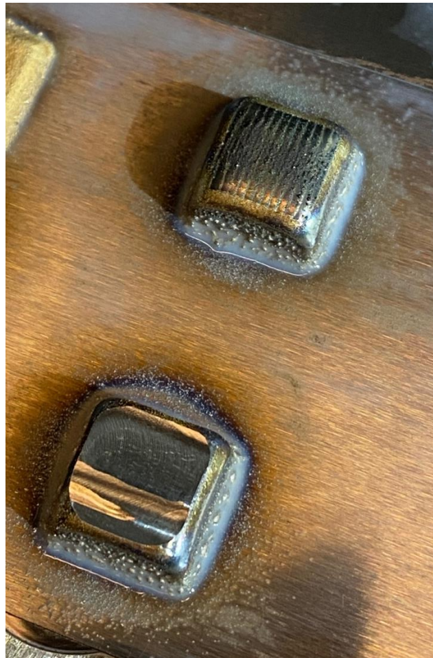
Figure 9. Example of fabrication process (Inconel 718): pre-facing specimen (top) and post-facing specimen (bottom).
