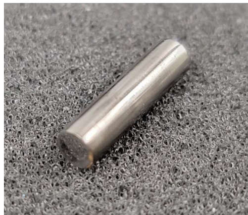
Figure 32. Constantan calibration sample (55%Cu, 45%Ni)
