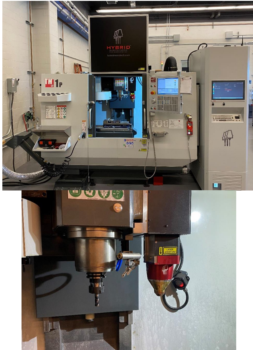
Figure 8. Hybrid Manufacturing Technology AMBIT DED Printer (top) and its components (bottom)
