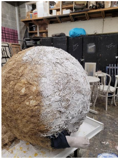
Figure 87: Coating with Elastomeric
