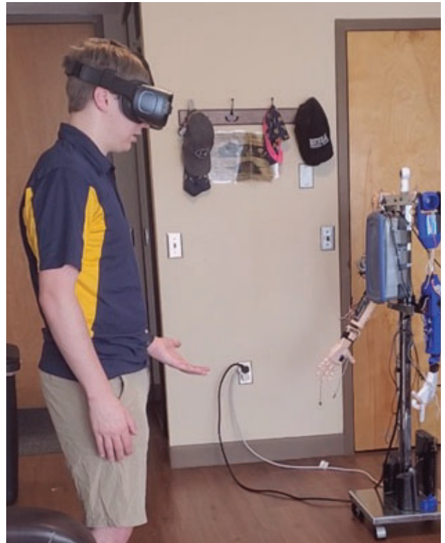
Figure 8. Gemini in Operation. Gemini mirrors the operator's hand moving up, while the operator views from the VR headset.
