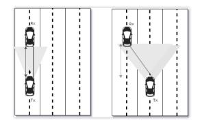
Fig.3. Communication between vehicles without light interference.
