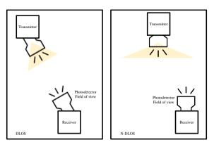
Fig.1. Illustration of communication channel model line of sight.
