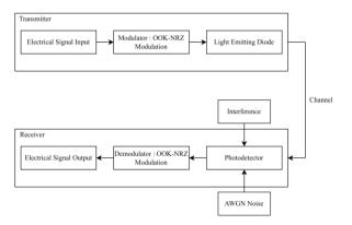
Fig.7. Diagram of communication systems between vehicles.
