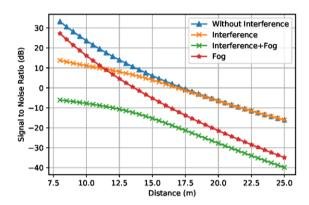
Fig.8. Comparison of various scenarios for SNR value.
