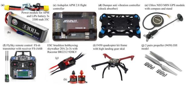
Fig. 4. Materials used for a drone with F450 frame and APM 2.8 flight controllers
