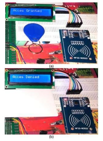
Figure 4 Display LCD: (a) Access granted and (b) Access denied
