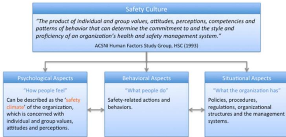
Figure 1 Safety Culture Abstraction (Developed by the United Kingdom’s Health and Safety Executive, 2005)
