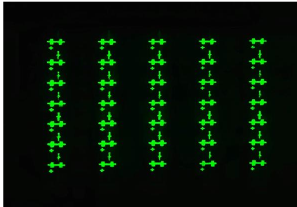
Figure 4-13 Image multiplication result at 532 nm
