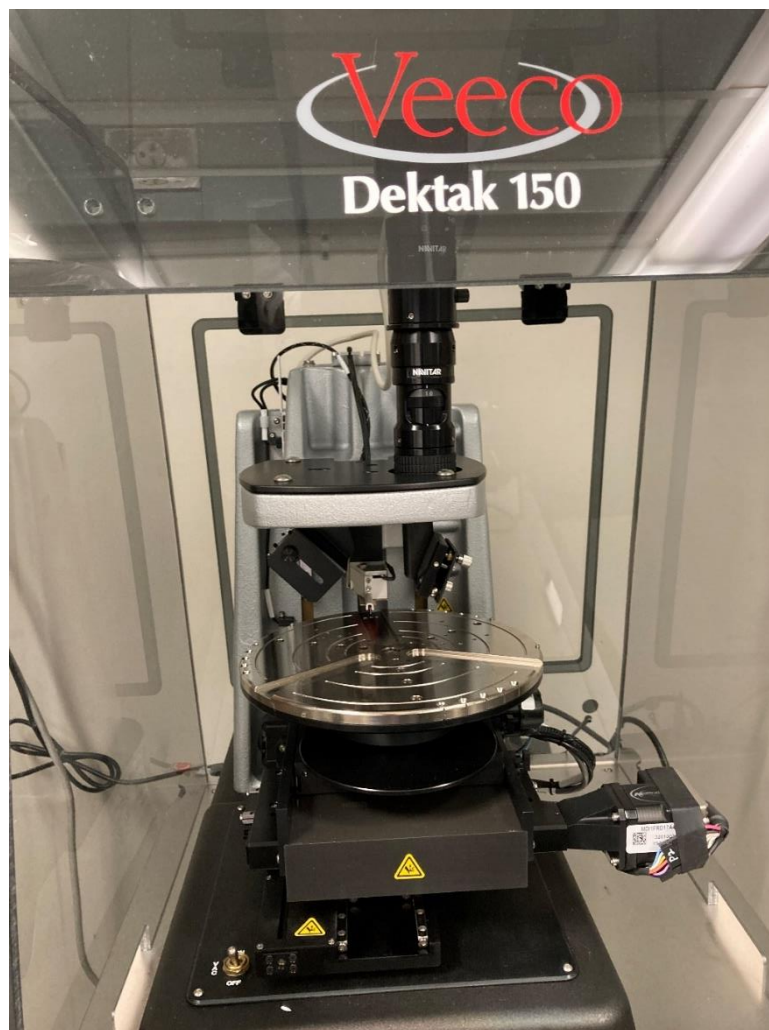
Figure 8: Dektak 150 Profiler to measure the thickness of the deposited thin film
