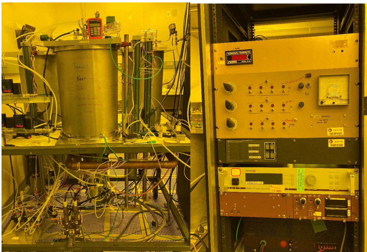
Figure 5: Custom built RF Sputtering, DC Sputtering, and Evaporation system
