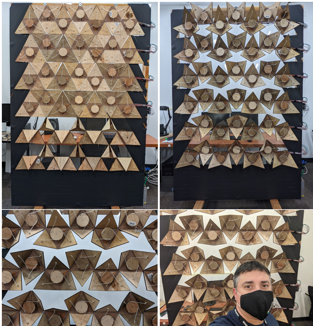
Figure 5.26: This figure demonstrates testing of the physical prototype in a lab space, which was accomplished one row at a time. Because the frame is larger than a typical doorway, it requires multiple people to move it to an actual experiment.
