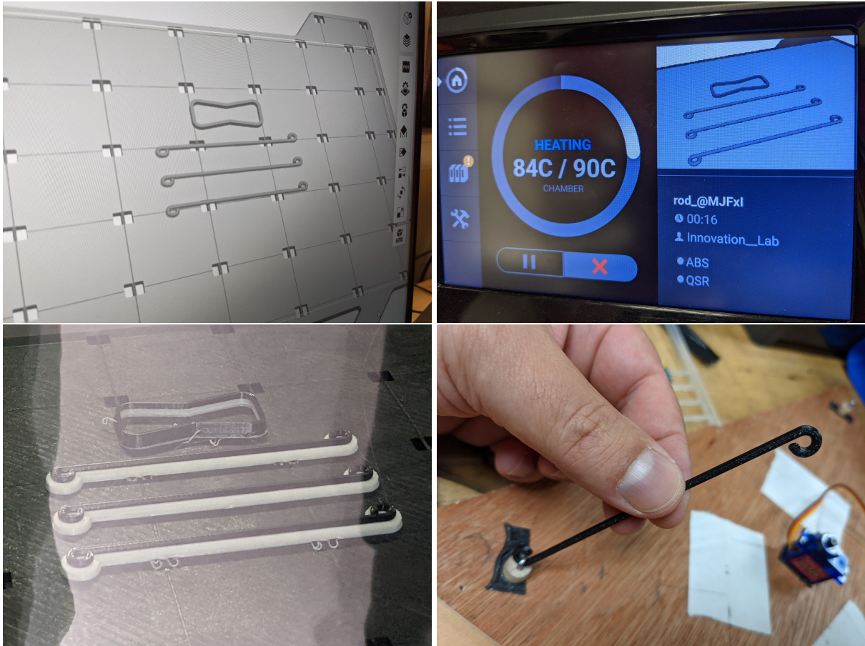
Figure 5.20: Here we show the 3D printing of triangular unit rods, which were perfect for the prototype because of their round shape and flexibility, but were too expensive to produce en masse.
