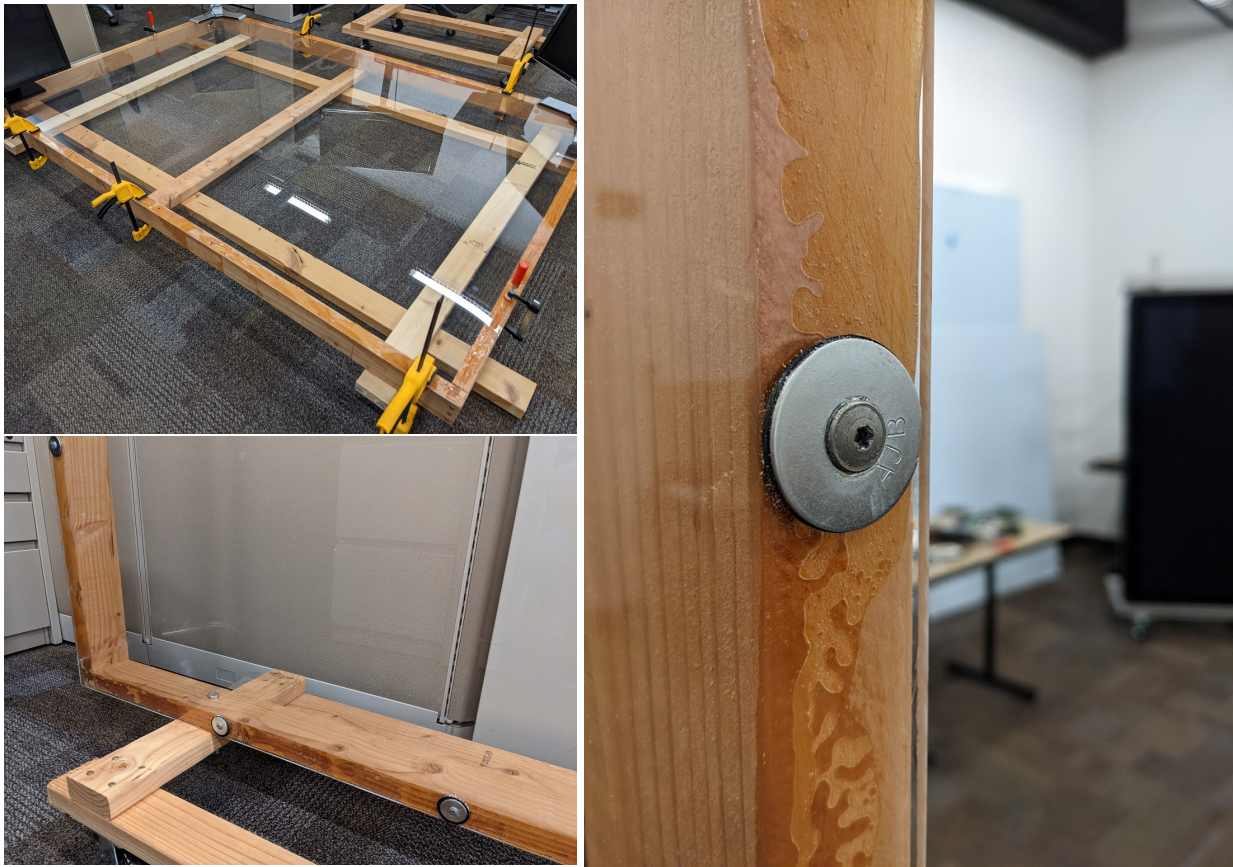
Figure 5.19: Here we show the 2 x 4 frame with mounted acrylic. The acrylic was both epoxied and screwed with star-drive deck screws pulling against neoprene and metal washers.
