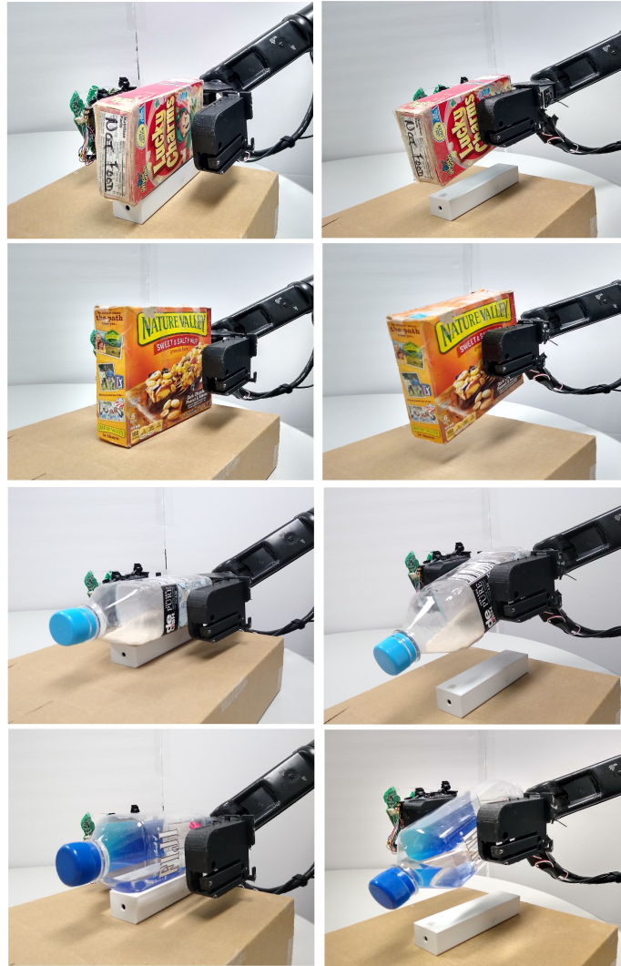
Figure 3.8: A side-by-side view of the grasped objects before and after closed-loop adaptive regrasping algorithm has been executed for predominantly rotational slippage.
