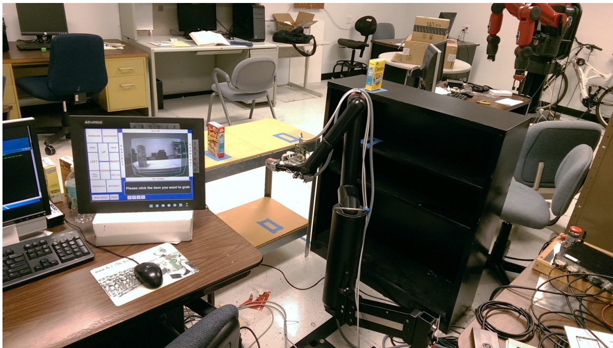
Figure 4.1: Setup of experiment with the UCF-MANUS was located to the right of the user, who controlled it with the mouse and the GUI displayed on the screen.[29]
