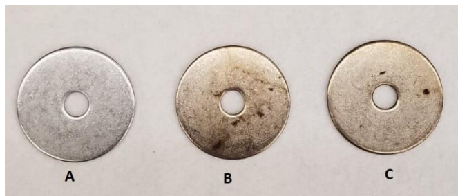
Figure 42: A visual comparison of coupons of 18-8 stainless steel kept at 350°C without hydrocarbon impingement (A) and after 200 pulses of cyclopentanone (B) and 2-methylfuran (C) impingement at 350°C.
