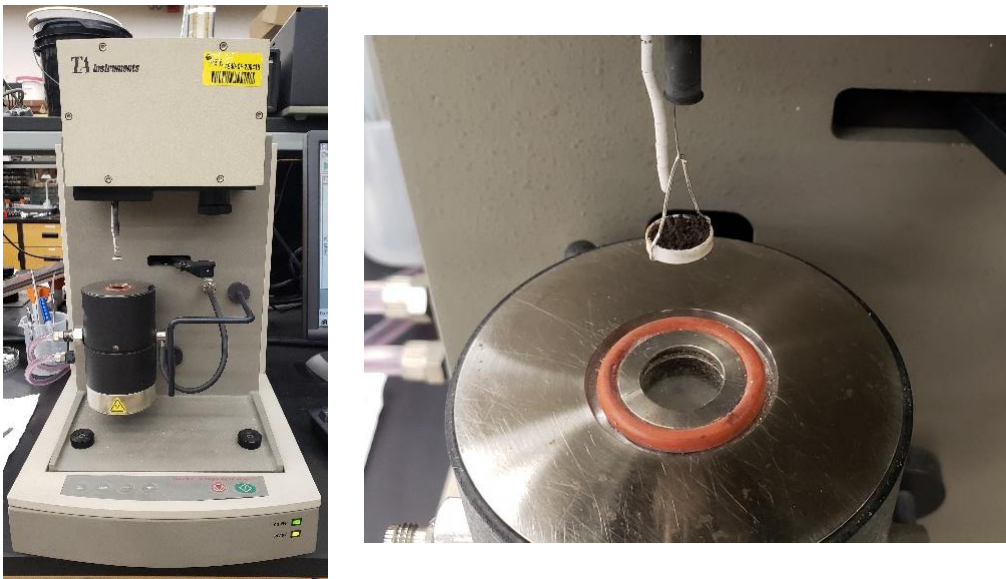
Figure 51: Thermogravimetric analysis (TGA) was used to monitor mass fluctuations of the pyrolants during ignition. The right image shows a sample of titanium and boron pyrolant mixture hanging on the weighing pan.
