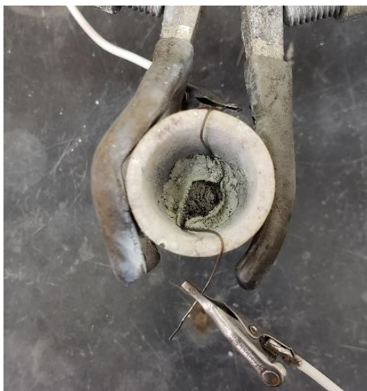
Figure 50: A post-combustion image of burned solid pyrolant in a ceramic crucible, atop a coiled nichrome wire. The reaction product has hardened around the wire coil.
