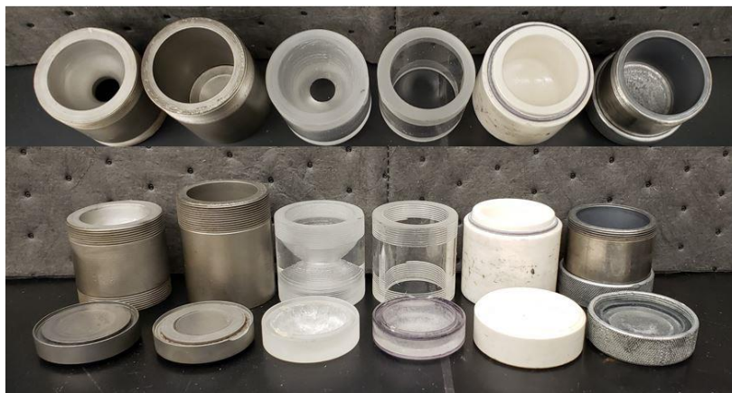
Figure 8: Mixer mill vials made from various materials (from left to right) stainless steel with “hourglass” interior, stainless steel, acrylic with “hourglass” interior, acrylic, zirconia, tungsten carbide. Top image is a top view of the vial interior.
