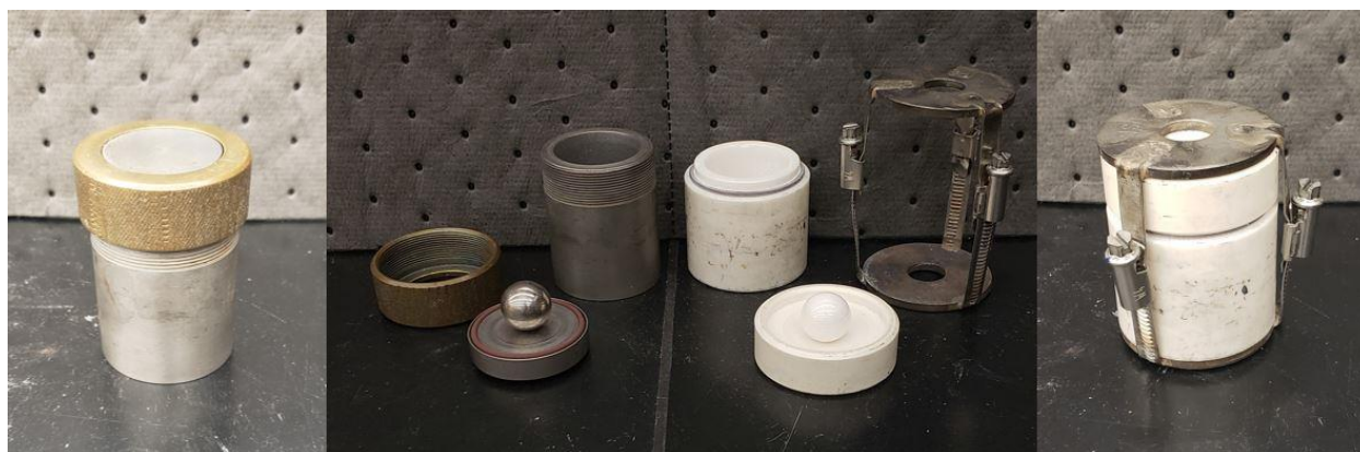
Figure 5: Shaker mill vials made out of stainless steel (left) and zirconia (right), both assembled and disassembled (disassembly in center). The stainless steel vial is sealed gas-tight using a screw cap (brass) while the zirconia vial uses a unique clamp to compress the lid down onto an o-ring located on the vial itself.
