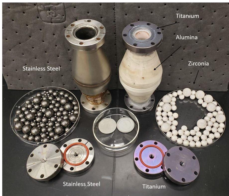
Figure 7: A stainless steel (left) and alumina (right) pebble mill vial, with their respective ball bearings. Two flanges (bottom) are used to close each end of the vial. Two filters (center in petri dish) are placed between the vial end and a flange on each side to prohibit reagents from exiting the reaction zone. O-rings (orange) seal the vial at the flange. Six bolts secure the flanges to the vial on each side. A threaded hole in the center of each flange accommodates for a gas inlet and outlet.
