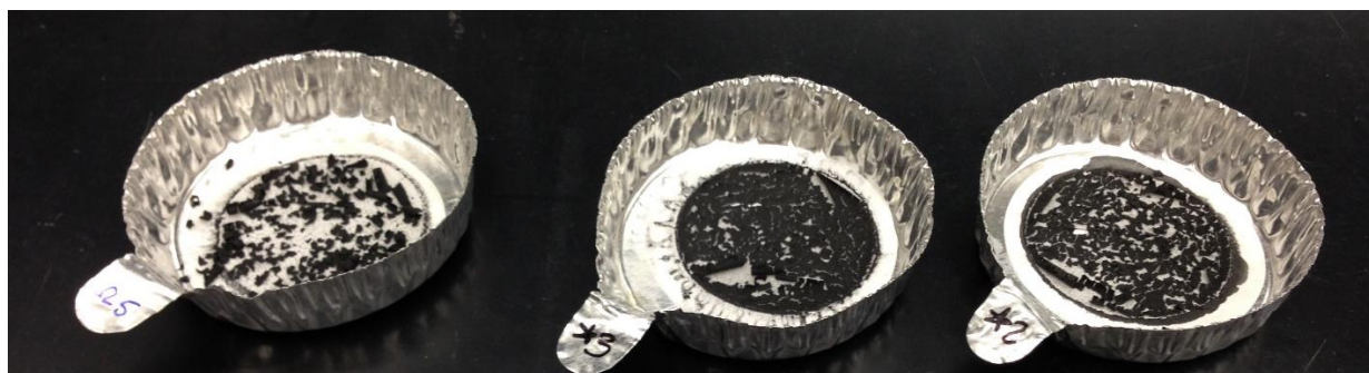
Figure 70: A mixture of δ-MoN and γ-Mo 2 N after washing and vacuum filtration.
