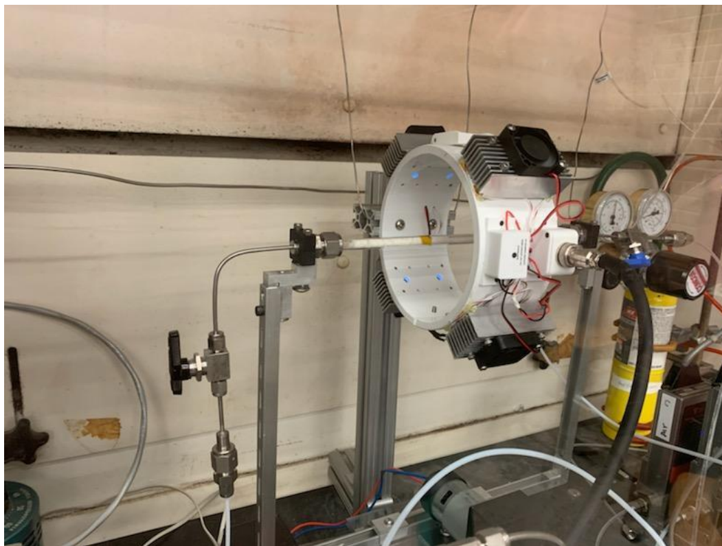
Figure 68: First iteration of a medium-intensity plug-flow photoreactor. The quartz tube contains dh -BN and is situated in the center of a circular light source.
