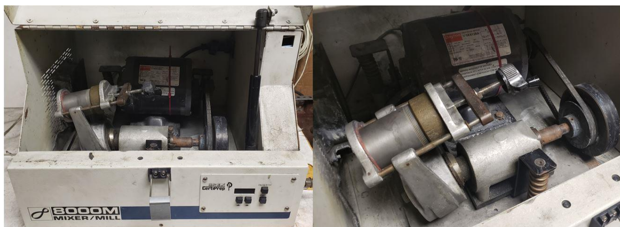
Figure 4: The shaker (mixer) mill with a clamped vial.
