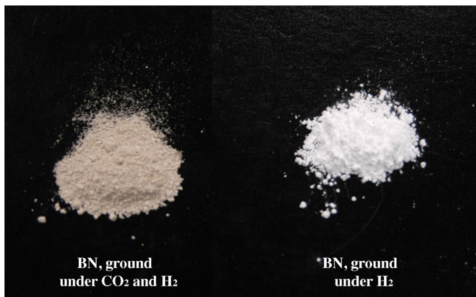
Figure 27: Defect-laden h -BN processed under H 2 and CO 2 produced low volatility side products that colored the catalyst. The same catalyst processed under hydrogen alone did not develop this color.
