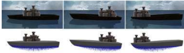
Fig. 9: Animation snaps of a boat with cargo distributed in different positions (above) and the corresponding pressure distribution exerted by the water (below)
