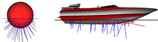
Fig. 5: Forces acting in a still ball and a moving boat (Blue arrows: buoyancy and lift forces, red arrows: drag forces).
