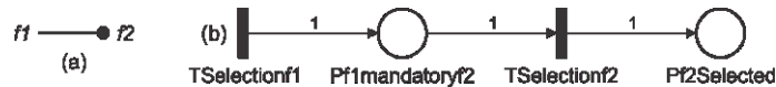
Fig. 2. Mandatory variability dependency. (a) FM including the mandatory feature ( f_2 ). (b) Proposed Petri net.
