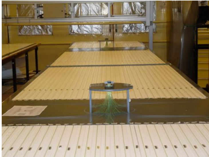
Figure 2: Two muon counters in the laboratory without their top PVC cover. In the middle of the counters are the ends of the 64 optical fibers and the connector to couple the fiber ends to the PMT.
