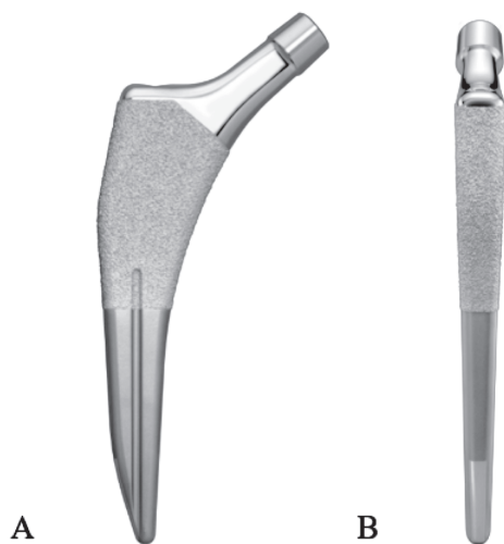
Fig. 1. Stem design. (A) Anterior view. (B) Lateral view. The Initia stem with a short tapered-wedge stem design allows for bone preservation and gradual load transfer from proximal to distal. The stem is also suitable for minimally invasive procedures because of its laterally reduced design, thin shape, and short length. This figure was provided by Kyocera Corporation, Kyoto, Japan.
