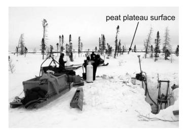
Fig. 2. The snow accumulation adjacent to the peat plateau at the Fletcher Lake site, April, 2007. The drill placed in the excavation marks the location of the snow bank thermistor cable (Fig. 9a). The surface of the bordering peat plateau is visible behind the trees.
