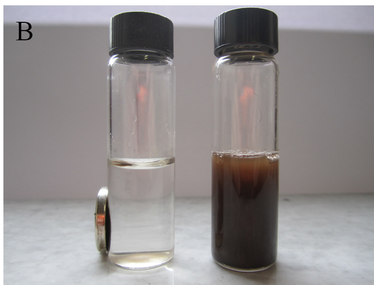
45 46 47 48 49 50 51 52 53 54 55 56 57 58 59 60 Figure 3. A) Magnetization curves of NP/0.5, NP/0.1 and NP/0.05 at 300 K. B) NP/0.5 dispersed in aqueous-solution and magnetic separation.
