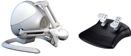
FIGURE 2: 3DOF Novint Falcon translational master device and 1DOF Genius rotational master device.
