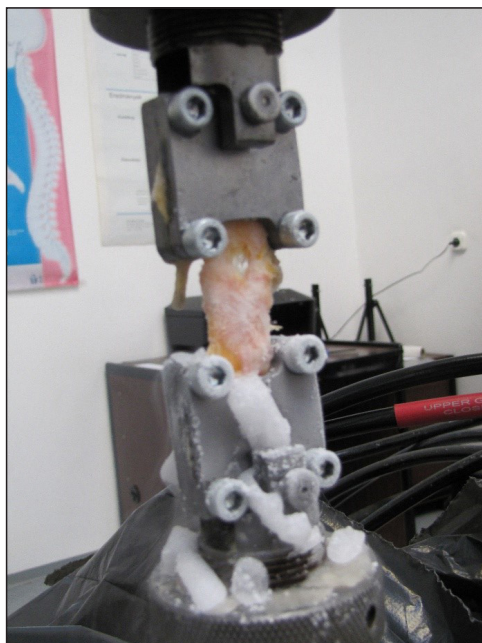
Figure 1. Test setup of the fatigue test
