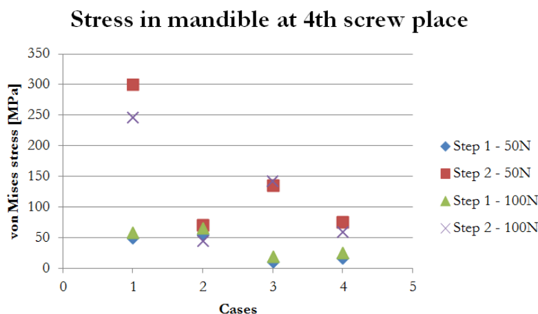
Figure 7. Different von Mises stress values at 4th screw place
