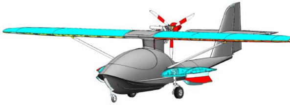
Fig. 1. A light amphibious airplane with a shock strut suspension.
