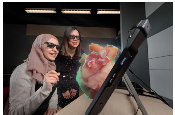
iEXCEL's Z-Space modules allow students to learn with advanced 3D Workbenches (pictured above). The users' vision is tracked by infrared cameras so that anatomical models are always viewed in full stereoscopic 3D. This technology allows students to manipulate and deconstruct models while studying and practicing their anatomical retention skills.
