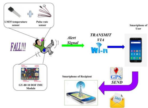
Fig. 1. Block diagram of the human fall detection system
