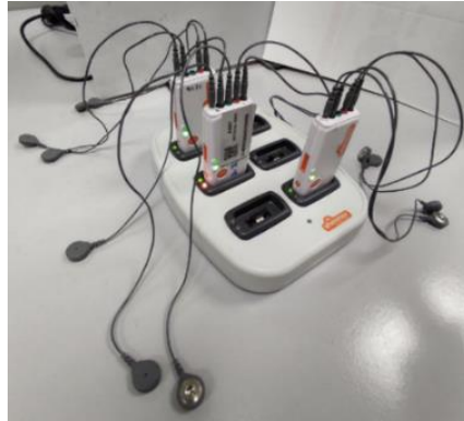
Figure 8: Installation Consensus Shimmer3 EMG Unit on Base6
