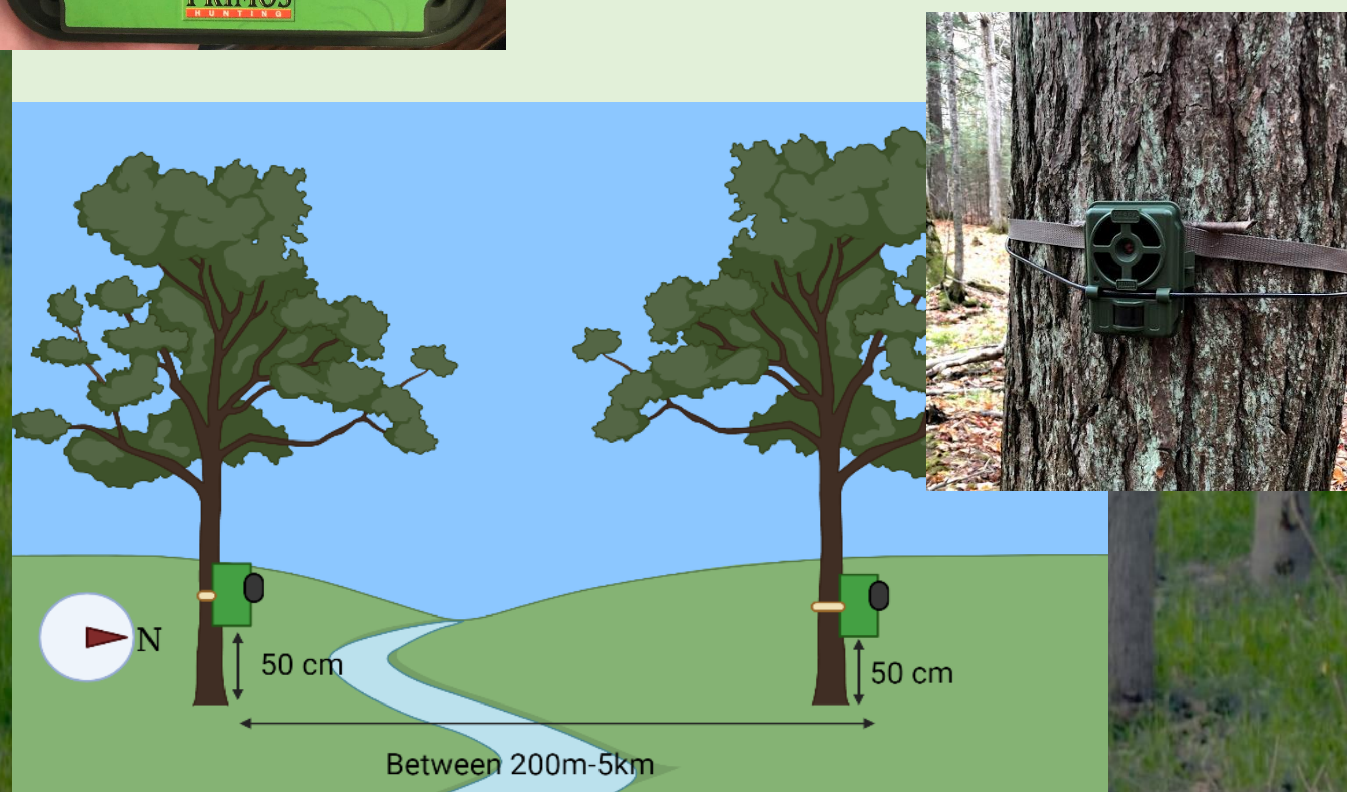
Figure 4 shows the setup of the camera traps. Each camera faced north, 50 cm from the ground and between 200m to 5km from other cameras. [8]
