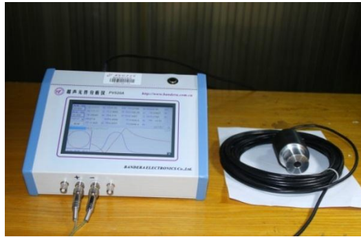
Fig. 3-10 A test platform based on impedance analyzer PV520A of SPUTs
