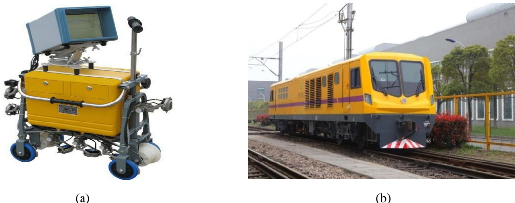
Fig. 1-2 The off-line detection equipment of rail flaw, (a) detection flaw trolley by hand push, (b) high-speed rail inspection vehicle
