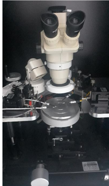
Figure 5.17. Photograph of the 4-point probe station located in the Complutense University of Madrid used for dark current-voltage measurements.
