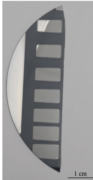
Figure 5.11. Photograph of an Al-based TLM contact deposited on silicon by RF sputtering.
