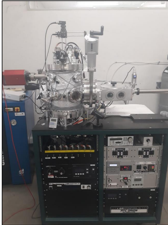
Figure 4.4. Magnetron reactive RF sputtering system used during this thesis at the University of Alcalá.
