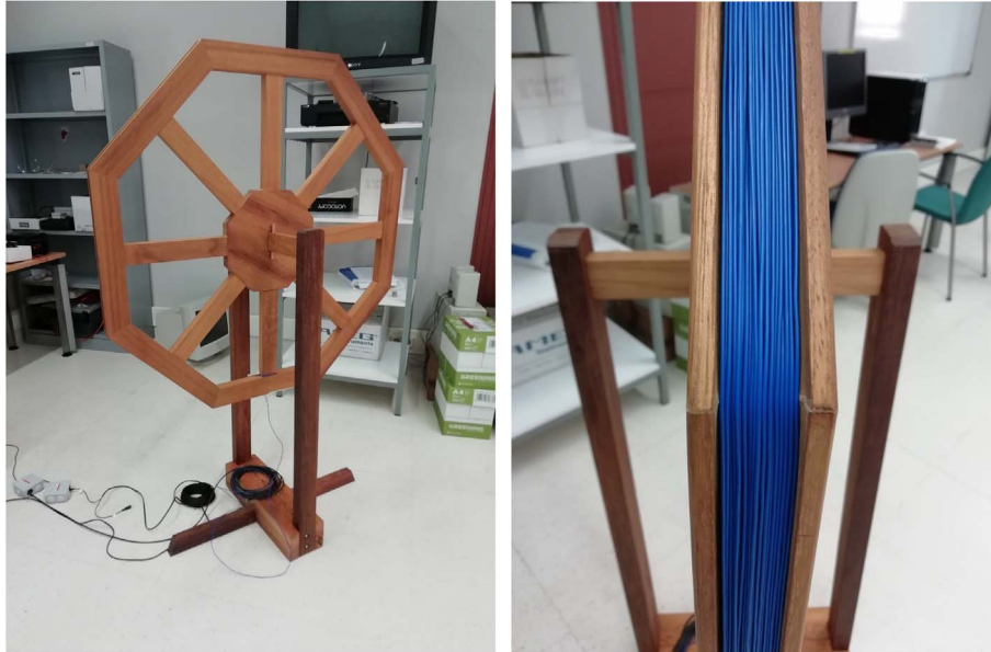
Fig. 1. Antenna structure with an octagon shape (left) and coil winding (right).
