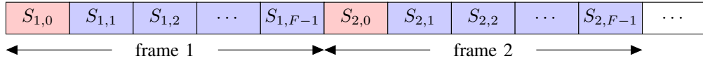
Fig. 2. Frame structure for the proposed DCT1e-based MCM scheme. Red boxes indicate the initial training symbol in each frame ( S_{i,0} with i denoting the frame number). Blue boxes indicate the remaining F - 1 data symbols ( S_{i,1}, \dots, S_{i,F-1} ).
