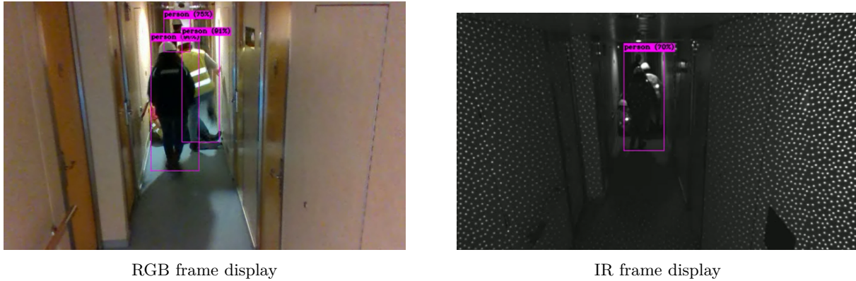
Figure 4.11: Difference between YOLO detection bounding boxes depending on the video recording setup
