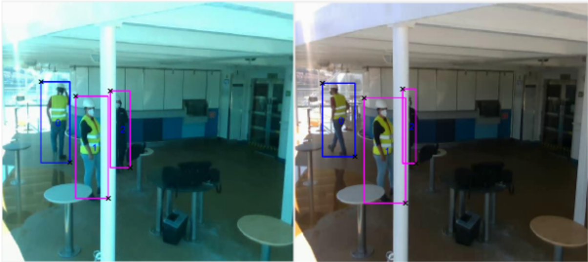
Figure 3.23: Walking action being labeled due to a displacement between frames from user 0
