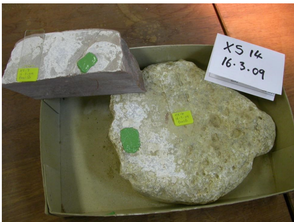
Figure 7: Lower stone XS14 made with of tuff and XS17 made of sandstone showing PVS Peel B series.
