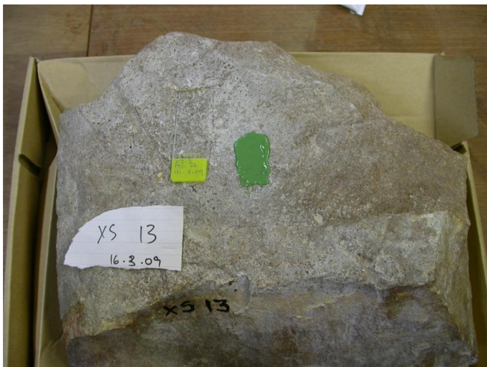
Figure 8: Lower stone XS13 made of sandstone showing PVS Peel A after cleaning and before use.
