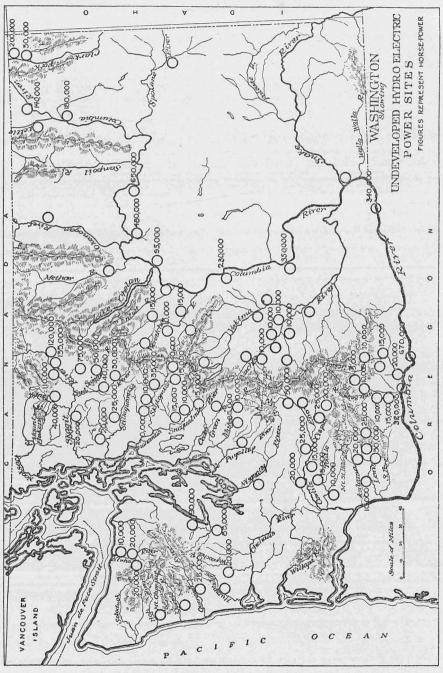
FIG. 2-Undeveloped Potential Power in Washington.
