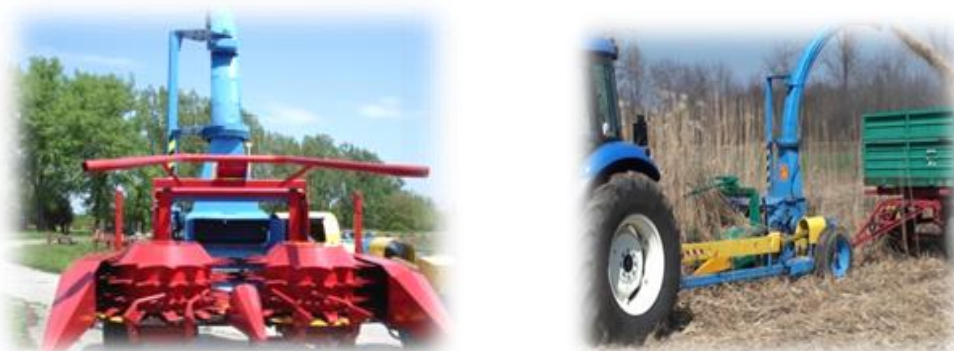
Fig. 9 - Towed combine for harvesting fodder CTF with the equipment for harvesting Miscanthus, [1,2,3,4]
