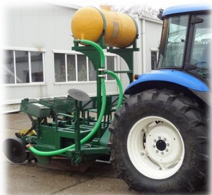
Fig. 4 - Installation for localized irrigation - IL-0, [1,2,3,4]
