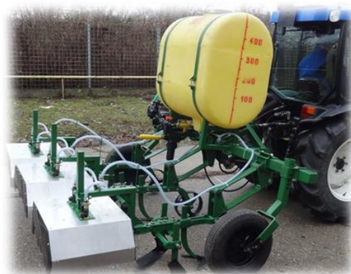
Fig. 5 – Equipment for precision hoeing and spraying in strips – MEP, [1,2,3,4]
