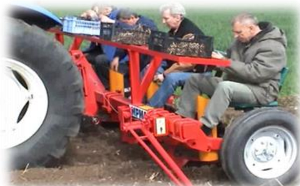
Fig. 7 - MPM4 machine for planting Miscanthus, [1,2,3,4]
