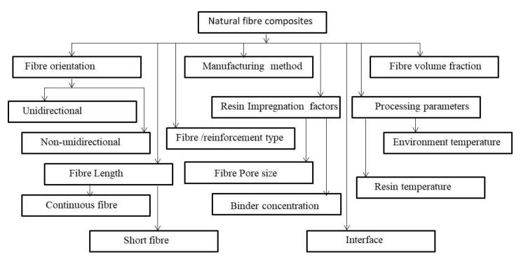
Figure 1: Factors affecting the properties of natural fibre composites adapted from [10,11]
