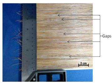
**Figure 3:** Coir fibres aligned without special means showing holes/gaps in-between the aligned fibres [29].
