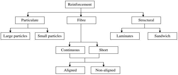
Figure 2: Various forms and orientations of reinforcements adapted from [27,28].
