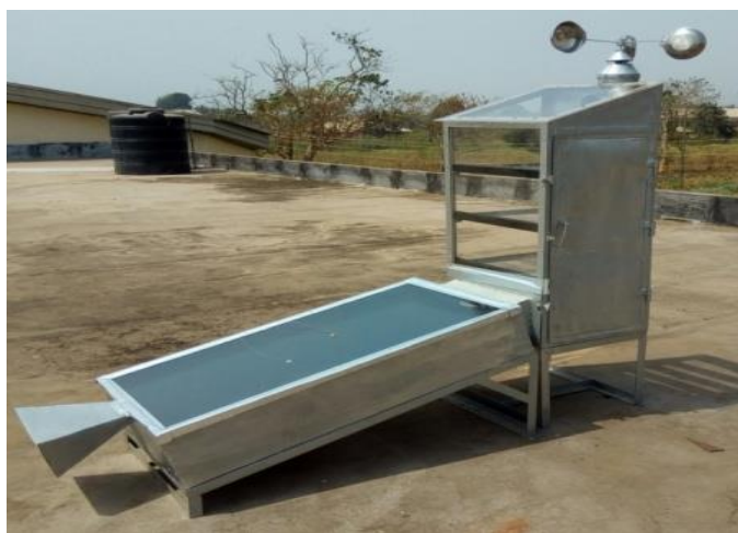
Figure 2: Fabricated Diagram of Mixed Mode Passive Solar Stock Fish Dryer
