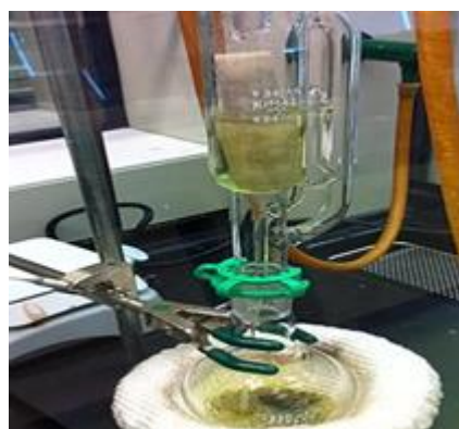
Fig 1: An Assembly of a laboratory soxhlet extractor
