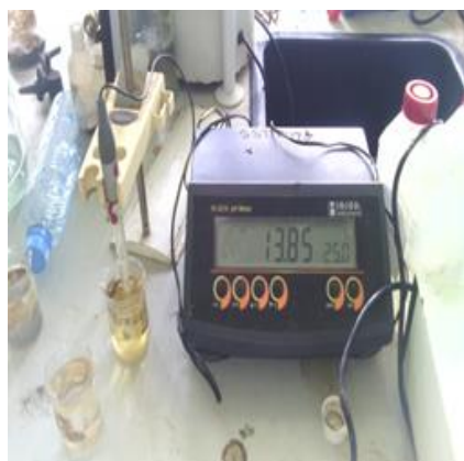
Fig3: pH Measurement of Test Media using HI 2210 pH Meter
