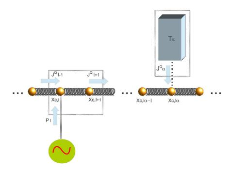
**Figure 2.** Sketch of the setup indicating the construction employed to derive the expressions for the heat currents as well as the poser developed by the external forces.
