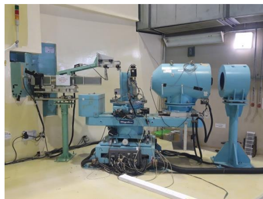
Fig. 1. The texture diffractometer (DN2).
