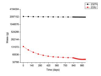
**Fig. 3(a)**. Mass depletion of the fuel isotopes (<sup>233</sup>U and <sup>232</sup>Th) in <sup>232</sup>Th-<sup>233</sup>U cycle.
