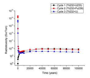
**Fig. 9.** Variation of the inhalation radiotoxicity, 100000 years after the fuel is discharge from the VHTR.
