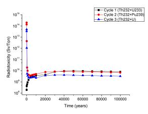
**Fig. 10.** Variation of the inhalation radiotoxicity, 100000 years after the fuel is discharge from the system VHTR+ADSs.
