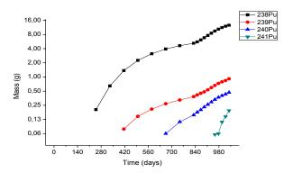
**Fig. 3(b)**. Plutonium isotopes variation in the hybrid system (<sup>238</sup>Pu, <sup>239</sup>Pu, <sup>240</sup>Pu and <sup>241</sup>Pu) in <sup>232</sup>Th-<sup>233</sup>U cycle.
