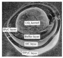
Fig. 2. TRISO coated fuel particle.
