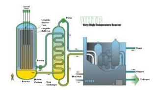
Fig. 1. Very High Temperature Reactor [3].
