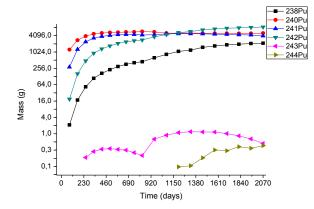
**Fig. 5(b)**. Plutonium isotopes variation in the hybrid system (<sup>238</sup>Pu, <sup>240</sup>Pu, <sup>241</sup>Pu, <sup>242</sup>Pu, <sup>243</sup>Pu and <sup>244</sup>Pu) in <sup>232</sup>Th-U cycle.
