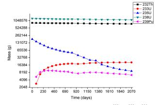
**Fig. 5(a)**. Mass depletion of the fuel isotopes ( $^{232}$ Th,  $^{233}$ U,  $^{235}$ U,  $^{238}$ U and  $^{239}$ Pu) in  $^{232}$ Th-U cycle.
