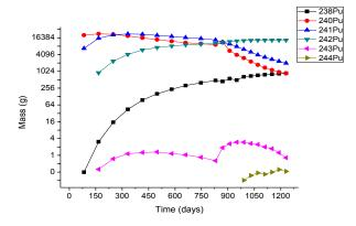
**Fig. 4(b)**. Plutonium isotopes variation in the hybrid system ( $^{238}$ Pu,  $^{240}$ Pu,  $^{241}$ Pu,  $^{242}$ Pu,  $^{242}$ Pu and  $^{244}$ Pu) in  $^{232}$ Th- $^{239}$ Pu cycle.
