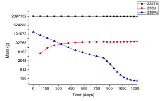
**Fig. 4(a)**. Mass depletion of the fuel isotopes ( $^{232}$ Th,  $^{233}$ U and  $^{239}$ Pu) in  $^{232}$ Th- $^{239}$ Pu cycle.
