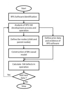
Fig. 3. Flowchart for the calculation of defects in the operation of RSG-GAS RPS software.
