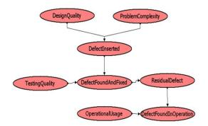
**Fig. 4.** A Bayesian network model for RPS software defects and reliability prediction.
