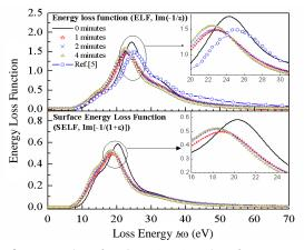
**Fig. 3.** Energy loss functions (ELF) and surface energy loss function (SELF) of  $\alpha$ -Al<sub>2</sub>O<sub>3</sub> in this study. These energy loss function described parameters in Table 1, which have been used as input to calculate the  $\lambda K_{th}$  values of Fig. 2. We have included the ELF from Ref. [5] for comparison.
