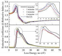
**Fig. 6.** Index of refractive (*n*) and extinction coefficient (*k*) of  $\alpha$ -Al<sub>2</sub>O<sub>3</sub> determined in this study. We have included index of refractive (*n*) from Ref. [5] for comparison.
