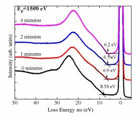
Fig. 1. Reflection energy spectra at energy 1.5 keV for  $\alpha$ -Al<sub>2</sub>O<sub>3</sub> as a function of sputtering times (as labeled).
