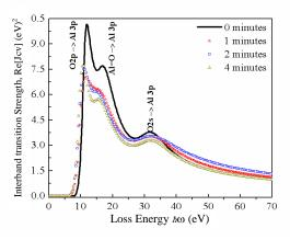
Fig. 5. Real part of Interband transition strength  $(J_{CV})$ .
