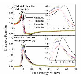
**Fig. 4.** Real part  $(\varepsilon_l)$  and imaginary part  $(\varepsilon_2)$  of dielectric functions of  $\alpha$ -Al<sub>2</sub>O<sub>3</sub> determined in this study.
