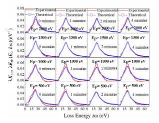
**Fig. 2.** Experimental inelastic cross section  $\lambda K_{exp}$  for  $\alpha$ -Al<sub>2</sub>O<sub>3</sub> (red line) obtained from REELS data compared to theoretical inelastic cross sections  $\lambda K_{th}$  (blue line) evaluated using the simulated energy loss function.
