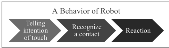
Fig. 1 Modeled Flow of Touch Performing by a Robot
