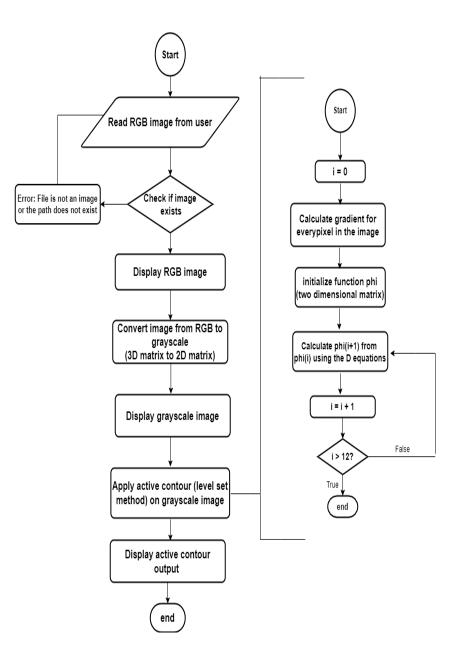
Figure 2: active contour flow chart
