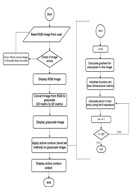
Figure 3: edge detection flow chart
