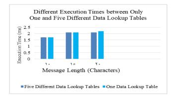
Figure 7: results chart of different messages encrypts with same password length using only one and five different data lookup tables
