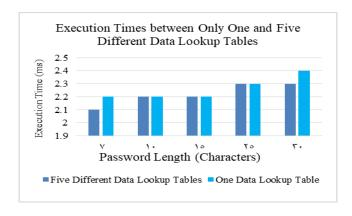
Figure 6: results chart of same messages encrypts with different password lengths using only one and five different data lookup tables.
